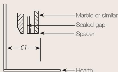
If your chimney has a shallow 'starter block' then use spacer kit 8315 and a 3" (75mm) deep rebate surround to achieve the C1 dimension. Pre-cast flues with a deep 'starter block' may be installed in exactly the same way as a conventional masonry opening providing there is a depth of 8½" (215mm) at C1.
